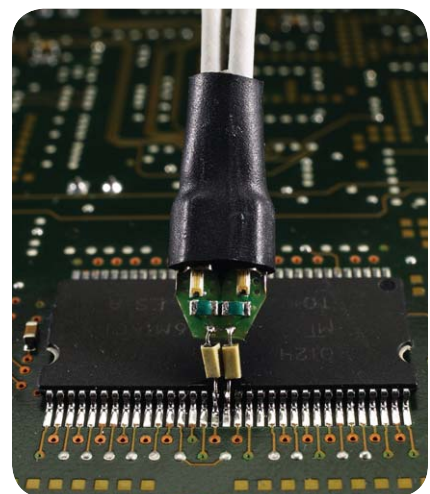
Figure 3. InfiniiMax solder-in differential probe head
