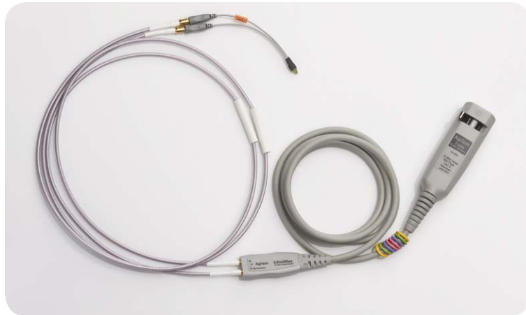
Figure 1 Probe head and extension cables connected to probe amplifier
