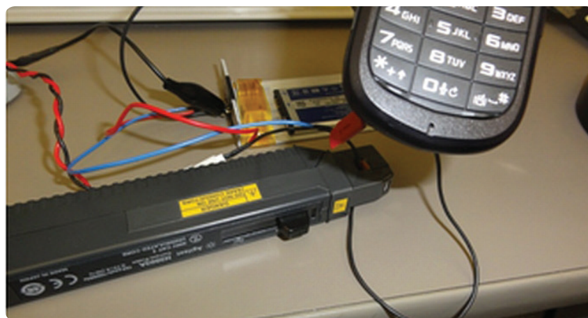
Figure 4-2. A simple way to measure a current with an oscilloscope is to use a clamp-on type current probe such as Agilent's 1147B or N2893A.
