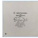
InfiniiVision scopes incorporate acquisition memory, waveform processing, and display memory in an advanced 1.3 micron ASIC. This patented 3rd generation technology, known as MegaZoom III, delivers up to 100,000 waveforms (acquisitions) per second with responsive deep memory always available.
