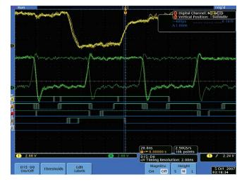
Figure 4. The Tek MSO4104 fails to capture the infrequent metastable state after 5 seconds of observation time.
