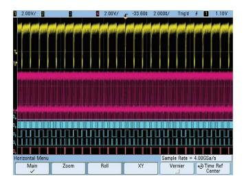
Figure 6. Although scaling the timebase to a slower range improves the probability that the MSO can capture the glitch, we are unable to visually "spot" the glitch on-the-fly while repetitively acquiring waveforms.
