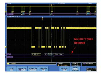
Figure 8. Tek's MSO4104 fails to capture and decode CAN error frames with a software-based decoding update rate of just one 1 decode every 5 seconds.
