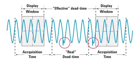
Figure 1. Oscilloscope dead-time versus display acquisition time.
