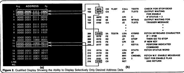
displays the address of the CALL instruction, 00F8. Therefore, during the next four machine cycles: the high-order 8 bits of the next instruction address are stored in the push-down stack; the low-order 8 bits of the next instruction address are stored in the push-down stack; the stack pointer is decremented by 2; and control is transferred to the first address of the subroutine.
