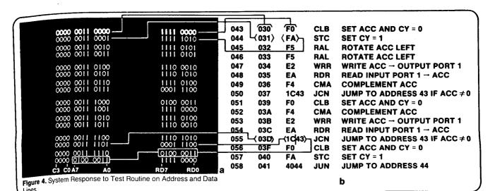
examined to show exact program operation. Note that line 14 of the state display corresponds to the first word of the JCN instruction at address 03D. The data in line 15 corresponds to the second word (0100 0011) of the JCN instruction, the address that program control is transferred to if the jump condition is true. Examination of line 16 reveals that the program did jump to the specified address.
