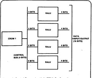
Figure 1. Central Processing Unit (CPU) Configuration
