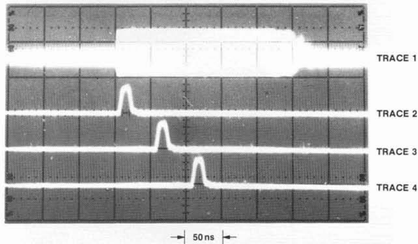
Figure 17. The scope photo shows an RF pulse and multiple exposures on the HP 5345A GATE OUT signal. The 20 ns gate is "walked" through the burst in 50 ns steps.
