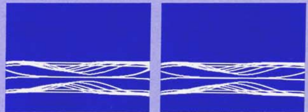
Figure 19. Shelving equalizer family of curves for two separate equalizers. 10 dB/vertical cm with horizontal reference times at \pm 10 dB and \pm 12 dB, log frequency sweep, 20 Hz to 43 kHz.
