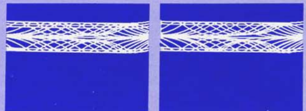
Figure 20. Peaking and notching curves for two separate equalizers. 10 dB/vertical cm with horizontal reference lines at \pm 10 and \pm 12 dB, log sweep, 20 Hz to 43 kHz.
