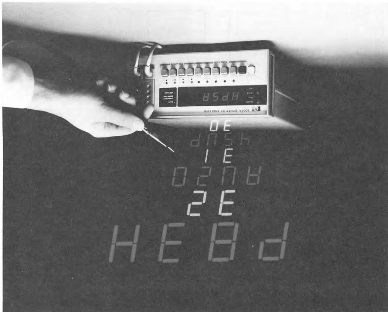
Figure 5. The operator can concentrate on probing without referring to the display using the signature memory in the HP 5006A. This makes misprobes and miscounts less likely. Time is saved when composite signature does not match because individual signatures do not need to be reprobbed. The memory can be reviewed in the RECALL mode by pressing the probe switch and then compared to printed tables.
