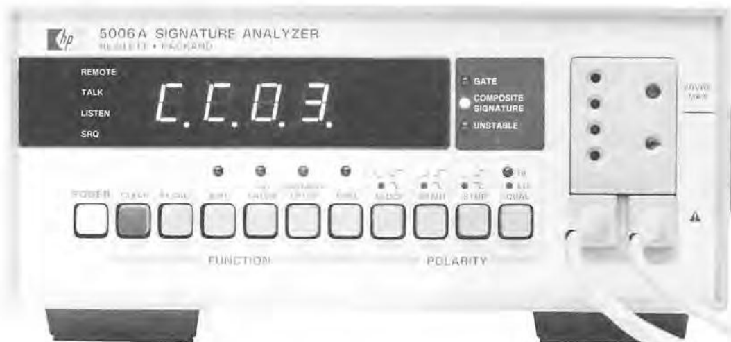
Figure 8. Troubleshooting is easier and faster with composite signature for those who do not have a computer-aided system. Composite signature is indicated in the RECALL mode with decimal points in the display and a lit LED between the gate and unstable LEDs just to the right of the display.
