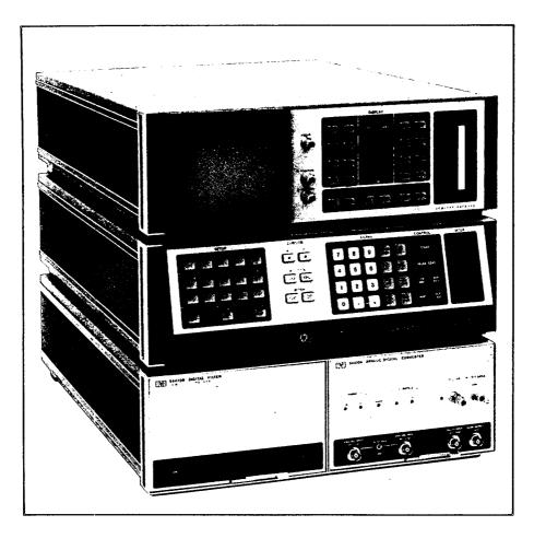
The Hewlett-Packard 5420A Digital Signal Analyzer utilizes sampled data techniques to perform a wide variety of single and dual channel measurements over a 25 KHz range. Measurements include Time Record Averaging, Auto and Cross Spectrum, Impulse Response, and Frequency Response. These measurements, and more, are described in Application Note 240-0.
