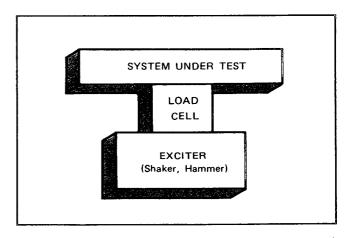
FIG 2. "IDEAL" MEASUREMENT SET-UP — Test system and exciter appear on separate sides of the load cell. Force sensed by load cell is the force actually applied to the structure.
