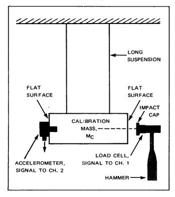
**FIG 8.** CALIBRATION MASS SYSTEM — The mass,  $M_c$ , should be large with respect to the accelerometer used. To determine the calibration curve, the mass is impacted along its center of gravity.
