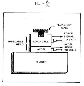
FIG 5. Test set-up used to measure effective mass of impedance head with loading mass. Resulting frequency response is  $H_{I}$ .
