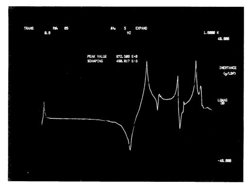
FIG 10. EFFECTS OF ACCELEROMETER LOADING — Accelerometer too massive — Black trace shows transfer function measurement with one accelerometer, White trace shows same measurement with accelerometer mass doubled. Comparison shows that this accelerometer was too massive for the disk brake structure under test.
