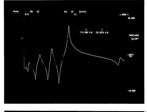
FIG 7. MASS LOADING EFFECTS — Impact Test System — White trace shows representative transfer function after compensation, Black trace shows uncompensated measurement. Note that mode frequencies and dampings are slightly lower because of mass loading, as indicated for the mode near 1 KHz.
