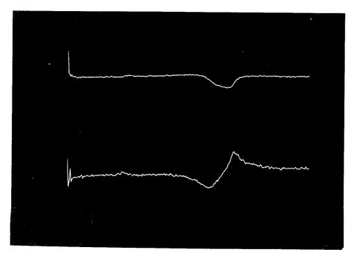
FIG 9.  $H_c$  FOR IMPACT TEST SYSTEM — Compensation curve calculated from calibration mass system.
