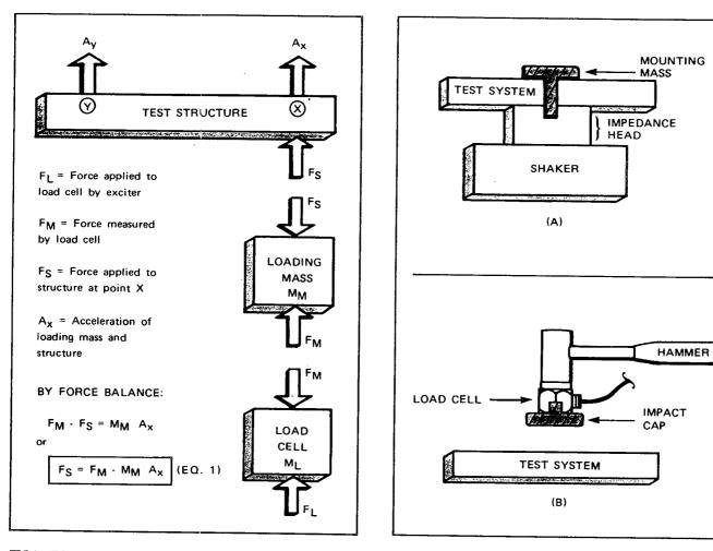
FIG 3. FORCES ACTING ON THE TEST SYSTEM — Equation 1 shows that the force actually applied to the structure is less than the force measured due to loading.
