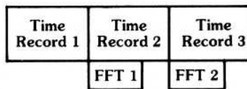
Figure 3.47 Real time operation
