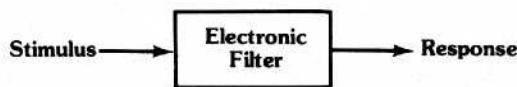
b) Electronic filter used to separate single conversation from FDM phone system
