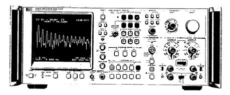
The HP 3582A is a spectrum analyzer covering the frequency range of DC to 25 kHz. Although it is a FFT-based, digital instrument, a special design effort has made it as straightforward to use as a conventional swept analyzer. With dual measurement channels it is possible to measure transfer function gain and phase, as well as the coherence function. A built-in random or pseudo-ran-
