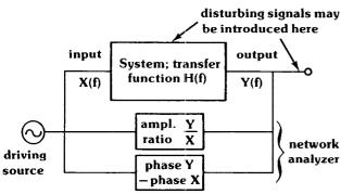
It is evident that determining the transfer function H(f) by calculating the spectral ratio Y(f)/X(f) will lead to irrecoverable errors whenever there is a disturbing signal included with the output Y(f). The 3582A reduces these errors through a computational technique: it uses the cross power spectrum (see appendix) and spectrum averaging. The question remains, however, how many averages are needed to attain a desired accuracy?
