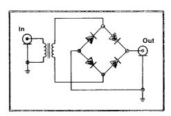
Figure 2. Typical frequency doubler circuit.
