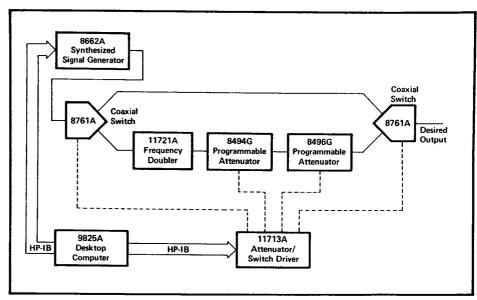
Figure 7. HP-IB System for convenient doubling control.
