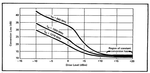
Figure 4. Typical 11721A conversion loss vs. drive level.
