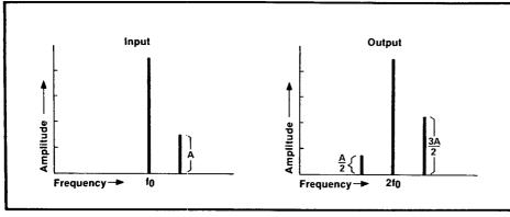
Figure 6. The effect of frequency doubling on spurious signals.
