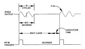
Figure 2. Parameters for programming a test signal burst
