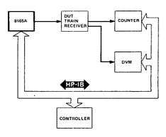
Figure 3. Test setup for train receiver
