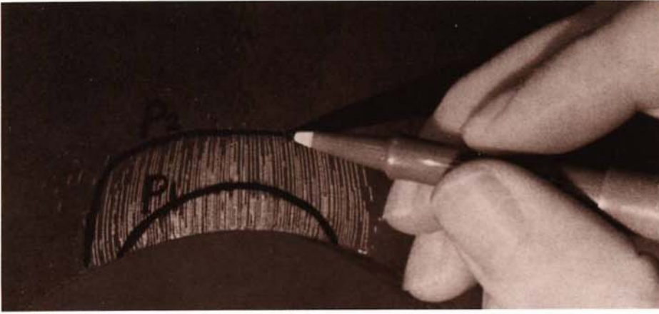
Figure 11 Cracks in a brittle coating Courtesy of The Photoelastic Division of The Measurements Group, Raleigh, North Carolina, U.S.A.
