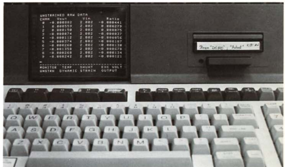
Display of a desktop computer used as instrumentation controller. Note the cassette tape on right used to store unstrained data (displayed).
