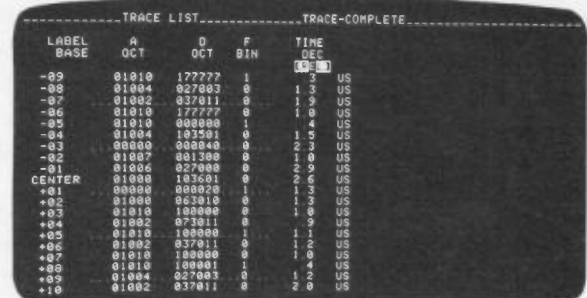
Figure 3. This Model 1610A list display shows address and data flow on an HP 21MX S-bus.
