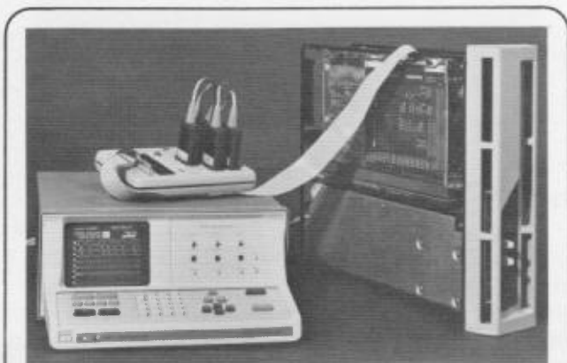
Figure 1. The powerful measurement set of today's logic analyzer is made possible by microprocessor control.
