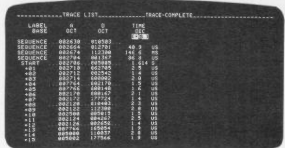
Figure 27. The trace list showing the relative measured times of execution for the routine of figure 25 shows the elapsed time between sequential states on the display.
