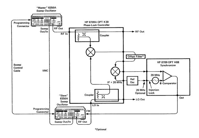
Figure 5. Two-tone System with Phase-Locked Offset Block Diagram
