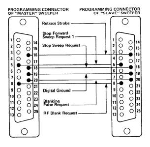
Figure 6. Sweep Control Cable Assembly
