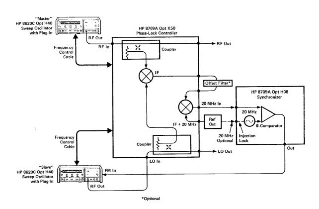
Figure 7. Two-tone Sweeping Generator Block Diagram
