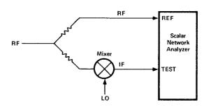
Figure 3. Mixer Conversion Loss Measurement
