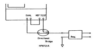
Figure 8. Measurement Setup (HP 4194A + HP 8721A)
