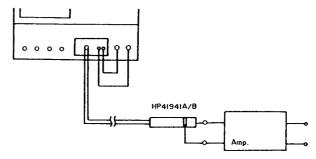
Figure 1. Measurement Setup (HP 4194A + HP 41941A/B)
