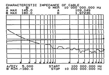
Figure 2 Sample Measurement Results (Characteristic Impedance)
