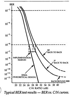
The purpose of C/N and C/I testing is to determine how a radio (or its modules) departs from the theoretical or design values. The test is also useful in the laboratory for optimizing and evaluating different implementations. Some typical BER test results are shown along with their representative theoretical curves.
