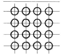
Constellation display of a 16QAM signal with an interfacing tone.
