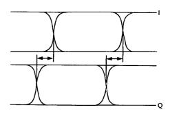
Time diagram of I/Q signals with data skew.
