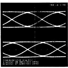
I/Q eye diagrams for offset QPSK.
