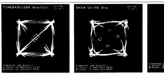
QPSK with no I/Q timing offset.
