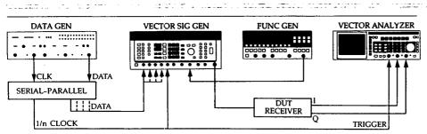
Complete AGC characterization can be done by simultaneously scalar modulating and digitally modulating the test signal.
