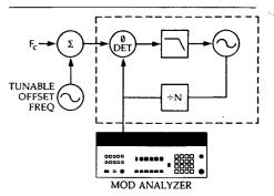
PLL test block diagram.
