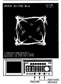
Measuring data skew of filtered signals with the vector analyzer.
