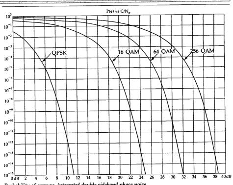
Probability of error vs. integrated double sideband phase noise.
