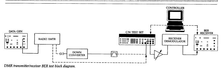
**Measurement Implementation** Configurations are shown for testing C/N of transmitters or back-to-back systems using the vector signal generator, the noise and interference test set and the BER test set. The HP 3708S Noise and Interference Test Set performs automatic measurements with HP-IB controllable BER testers. The measurements can also be made manually with a wide range of nonprogrammable BER testers.
