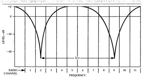
Frequency spectrum of a multipath fade.
