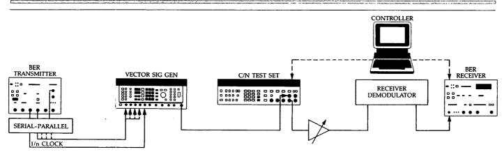
DMR receiver only BER test block diagram.
