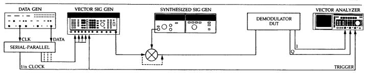
Vector demodulator test block diagram.
