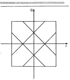
Vector diagram of QPSK with data skew.
