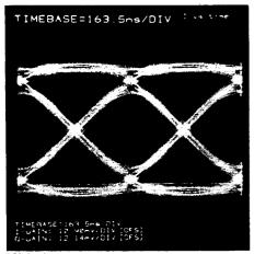
*ISI is the spreading of the symbol levels at the clock instant.*
