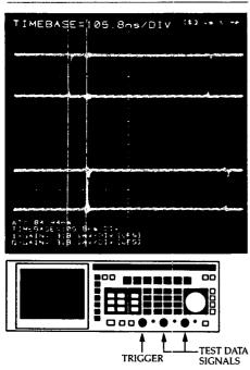
Measuring data skew of unfiltered signals with the vector display.
