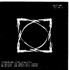
QPSK with 1/2 clock period I/Q timing offset.
