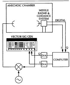
Figure 34. A closed hardware-in-the-loop test system. The HP 8780A Vector Signal Generator provides the l/Q modulator which allows the amplitude, phase, and frequency of the signal to be varied. The computer continuously calculates the Doppler shift, time delay, and amplitude of each pulse in terms of 1 and Q modulating signals.
