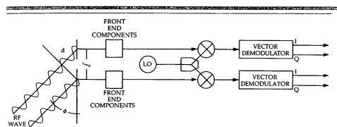
Figure 30. Phase monopulse. When a target return is off boresight, the extra distance traveled by one channel causes a phase difference.
