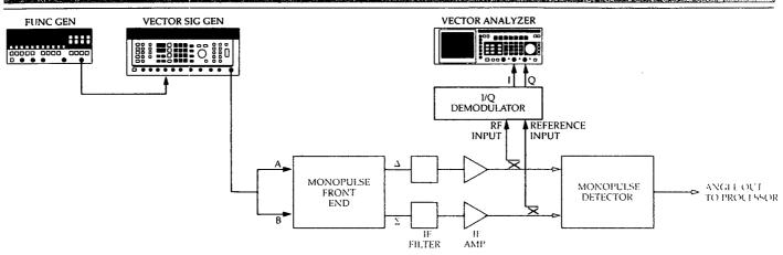
Figure 29. The vector measurement system here tests the phase matching of the sum  $(\Sigma)$  and difference  $(\Delta)$  channels.
