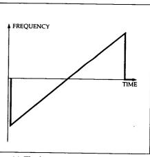
Figure 15. Plots related to the chirped signal in Figure 14. The frequency plot was calculated by taking the derivative of the phase plot. The phase plot was derived from I and Q.
