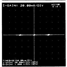
Figure 12. The vector diagram of a phasecoded pulse. The three states are displayed along with the trajectory paths taken between states. These paths indicate the signature of the
