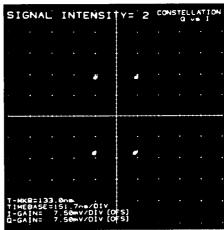
Figure 20. A QPSK signal will appear as a rectangle for gain mismatches in the I and Q channels.
