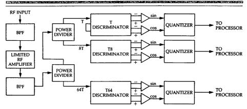
Figure 32. Digital instantaneous frequency measurement (DIFM) receiver.
