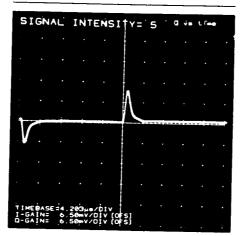
Figure 6. The l and Q channels versus time for the simple pulse in Figure 3.
