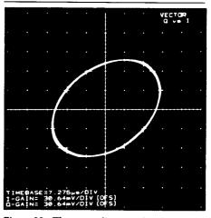
Figure 23. The vector diagram of a frequency offset will change from a circle to an ellipse when there are gain and phase quadrature errors in the demodulator.
