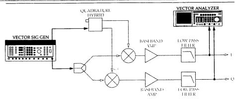
Figure 18. Calibrating a vector demodulator. The HP 8780A Vector Signal Generator inputs a test signal while the HP 8980A Vector Analyzer displays quadrature, gain, and dc errors. The demodulator can then be adjusted while watching the result on the vector display.
