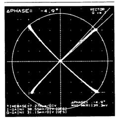
Figure 25. As the input power to the receiver is increased, gain compression and phase shifts occur. These errors can be easily measured with the magnitude and phase markers of the HP 8980A Vector Analyzer.
