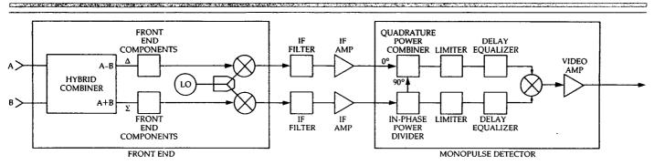
Figure 28. This monopulse receiver converts the amplitude measurement of the two channels into a phase measurement for processing.
