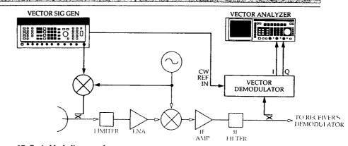
Figure 17. Basic block diagram of a vector measurement system and receiver. Just the receiver RF and IF sections are being tested.
