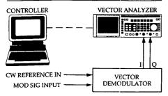
Figure 2a. This section of a vector measurement system can analyze a signal by breaking it down into quadrature components. The system reveals the signal's phase and amplitude.
