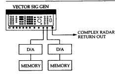
Figure 27. This system could potentially simulate different environmental radar returns. Possibilities include clutter returns, target returns, glint and scintillation effects.
