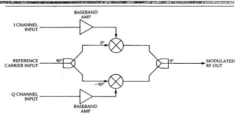
Figure 5a. A vector modulator synthesizes a complex modulated signal from baseband I and Q inputs and a CW carrier input.
