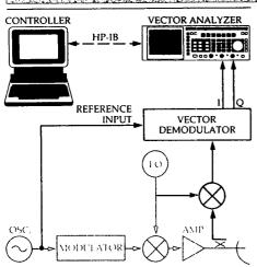
Figure 10. Vector measurement system for testing a transmitter at RF. The system will perform signature analysis of the signal's modulation.
