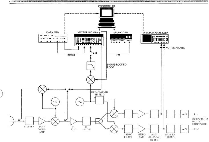
Figure 16. A vector modulation test system connected to a superhetrodyne receiver. The vector signal generator inputs a signal and the distortion caused by travelling through the receiver is analyzed with the vector display and a computer.
