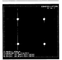
Figure 19. A QPSK signal on a vector display. The clusters form a square indicating the demodulator is in quadrature. The corners of the square determine the different signal states when the pulse is on. The lines represent the transitions between states.
