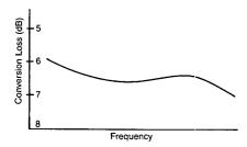
Figure 1a. Plot of mixer conversion loss, i.e. IF power relative to RF input power as a function of frequency.
