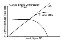
Figure 1d. Plot of conversion loss and IF output power as a function of RF input power level as normally shown on the scalar analyzer. Note that the !F output power increases linearly with the increasing RF signal, until mixer compression begins and the mixer saturates.
