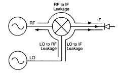
Figure 1e. Diagram showing the signal flow in a mixer. Note that RF and LO feedthrough signals may appear at the mixer IF output, together with the desired IF signal.
