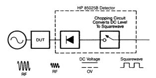
Figure C. DC detection detects unmodulated RF, then chops the detected signal. The receiver thus measures the desired signal, plus any other signals present at the detector.
