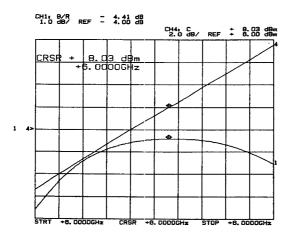
Figure 8. Plot of mixer conversion loss as function of LO input power level. Note that the conversion loss decreases until the optimum LO drive level is reached, and then increases as the mixer compresses at high LO drive levels.
