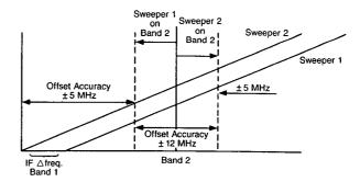
Figure 4. Representation of the frequency errors induced when the two sweep oscillators are on the same frequency band  $(\pm 5 \text{ MHz})$ , and when the sweep oscillators are on different bands  $(\pm 12 \text{ MHz})$ .
