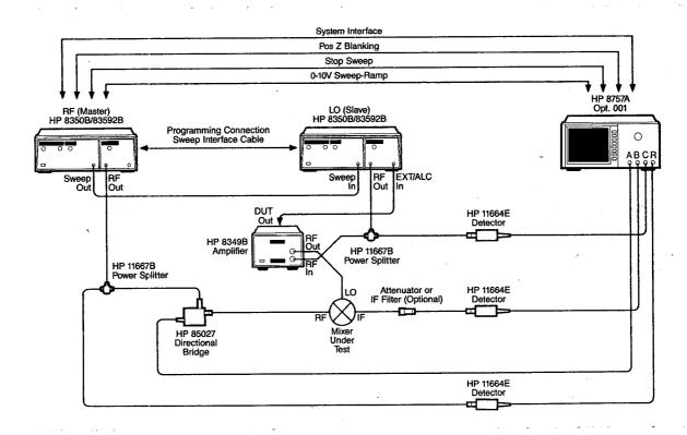
Figure 2. Setup diagram for measurements of mixer conversion loss, conversion compression, and RF input return loss. The amplifier is optional, and can be used to provide LO drive levels of up to +20 dBm.
