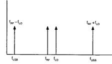
Figure 1b. Spectrum of RF, LO and IF signals present in mixer measurements.
