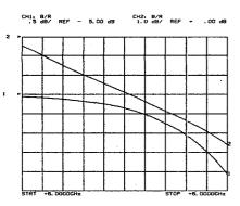
Figure D. Plot of mixer conversion compression measured using the HP 85025B detectors in DC mode. Trace 1 shows the characteristic compression of the mixer because a low-pass filter is used at the IF port to eliminate LO feedthrough. Without filtering of the IF, the measurement is invalid, because in DC detection mode, the sum of the IF and LO feedthrough signals is measured by the analyzer (trace 2).
