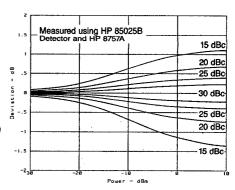
Figure G. Worst case power measurement uncertainty in the presence of second harmonics of different levels, as a function of fundamental power level at the detector. For example, for an IF signal at -10 dBm, and a second IF harmonic at -20 dBc (-30 dBm), the error is  $\pm 0.4$  dB. Note that for power levels below -20 dBm, the error is minimized.
