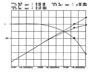
Figure 7. Plot of a 1-dB conversion compression measurement. This test is performed at fixed frequency, with the RF sweep oscillator in power sweep mode. Trace 1 shows the conversion loss (IF relative to RF), trace 2 the IF output power, and trace 3 shows the RF input power.
