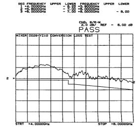
Figure 10. (a) Example limit entries for the maximum conversion loss conversion specification and (b) plot showing the limit lines, conversion loss trace, and PASS/FAIL status.
