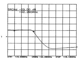
Figure 6. Plot of mixer conversion loss as a function of IF frequency (swept IF conversion loss). With this technique, IF mixer bandwidth and flatness can be characterized.
