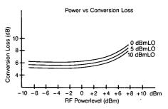
Figure 1c. Plot of a typical mixer's conversion loss as a function of RF input power level. The different traces show that conversion loss decreases when the LO signal power level is increased.
