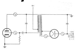
Figure 1. Typical RF Oscillator Used for an Oscilloscope Beam Supply
