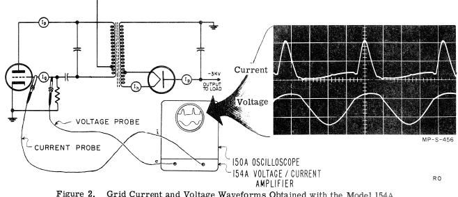
Grid Current and Voltage Waveforms Obtained with the Model 154A
