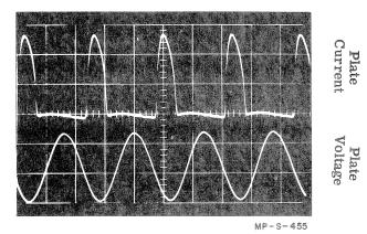
Figure 3. Waveforms Obtained With 154A
