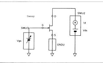
Figure 19. K, V<sub>TO</sub> Measurement Circuit
