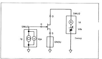
Figure 21. R<sub>s</sub> Measurement Circuit
