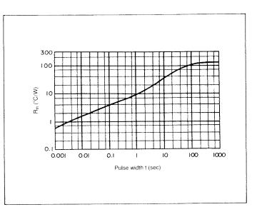
Figure 6. R<sub>th</sub>-t Pulse Width Curve
