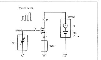
Figure 35. R<sub>ON</sub> Measurement Circuit
