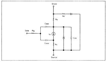
Figure 30. Power MOSFET Circuit Model
