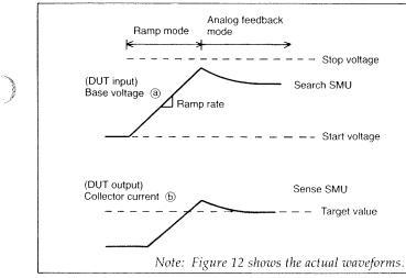
Figure 8. AFU-Related Waveforms
