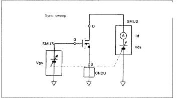
Figure 31. K, V<sub>T</sub> Measurement Circuit
