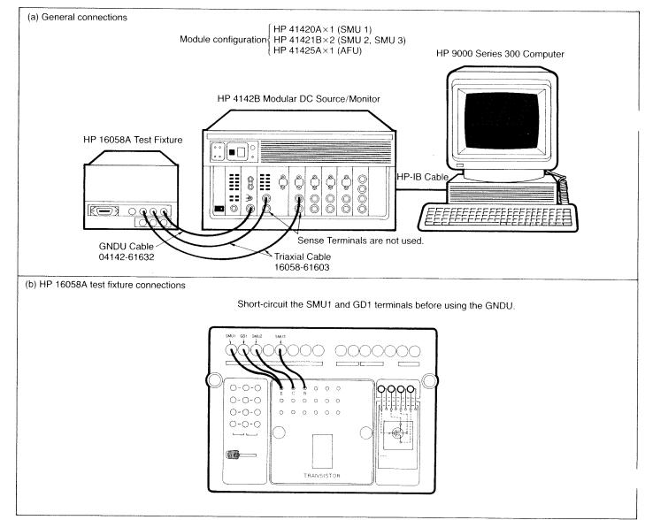
Figure 16. Test Fixture, DUT, and Controller Connections
