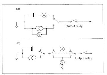
Figure 2. SMU Equivalent Circuit
