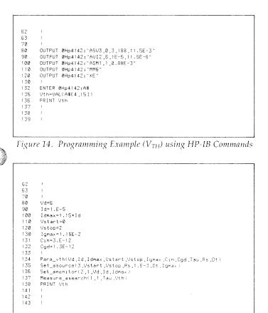
Figure 15. Programming Example (V<sub>TH</sub>) using Furnished Subprograms
