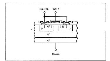
Figure 29. Power MOSFET Structure
