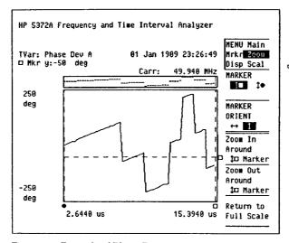
Figure 11. Example of Phase Deviation measurement with incorrect carrier frequency.
