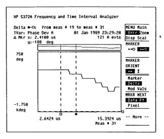
Figure 14. Using the markers in delta mode, you can determine the phase shift at each step in the code.
