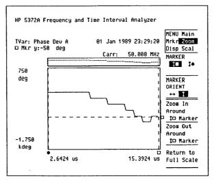
Figure 13. This plot of phase versus time shows the cumulative progression of phase through the Barker code
