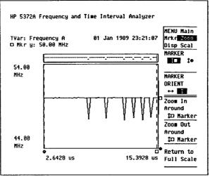
Figure 8. Positioning the  $1 \square$  marker to estimate carrier frequency.
