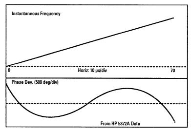
Figure 10. Result of fitting a parabola to the data and computing the difference.
