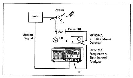
Figure 2. Typical equipment setup for measuring a chirped radar pulse.
