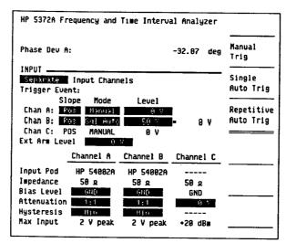
Figure 6. The completed INPUT menu shows the appropriate trigger threshold settings for Channel A and External Arm.
