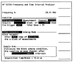
Figure 5. The completed FUNCTION menu shows selections for measurement type, block size, arming and sampling.
