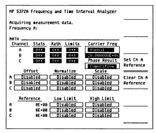
Figure 8. The MATH menu after entering carrier frequency and specifying type of phase display.
