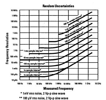
Figure 3. Frequency resolution depends primarily on sample interval and measured frequency.
