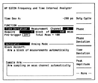
Figure 5. You can select the arming mode after moving the highlight (with the cursor keys) to the Arming Mode field. Here Interval Sampling is selected.
