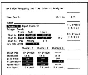
Figure 6 - To set up the input channel hardware, press the Input hardkey, and this screen appears. Here select a Positive going edge on Channel A with the trigger level set manually at 800 mV.
