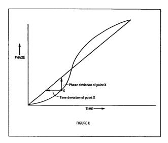
Figure C. Jitter is defined as a digital signal's deviation in time from its ideal position. Phase modulation looks at the signal's deviation in phase from its ideal.
