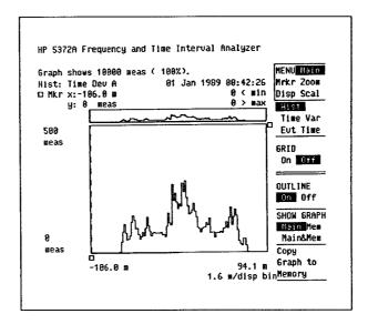
Figure 19. The histogram allows you to visualize the variability of jitter measured over some extended period of time. Use the cursors to quantify any bin value.
