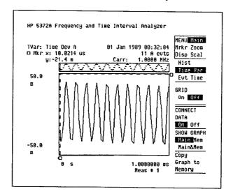
Figure 9. A view of the jitter is first enhanced with a connectthe- dots capability. Adding a grid may also help.
