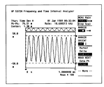
Figure 1. Jitter as a function of time. You could call this a jitter oscilloscope. For a strong periodic element of jitter, frequency is displayed as well as peak-peak jitter in Unit Intervals.
