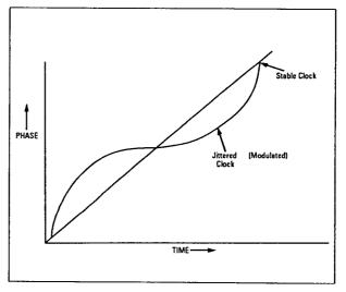
Figure B. A stable non-jittered clock's phase is a linear progression with time, whose frequency is  $\triangle$  phase  $/\triangle$  time. A jittered clock's phase progression is non-linear.
