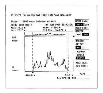
Figure 20. You can use the Stats function to calculate peak, mean and standard deviation of the data that is between the cursors.
