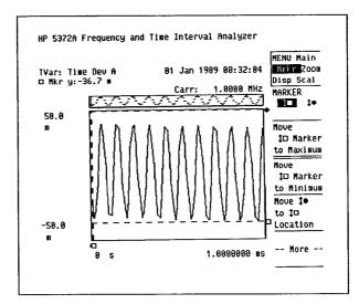
Figure 10. The Markers further enhance analysis. First move the  $\square$  marker to the minimum of the waveform.
