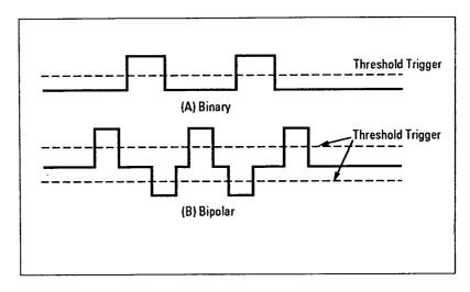
Figure 2. The threshold (trigger) on the HP 5372A (a) is set at the 50% point on a binary signal and (b) at the 50% of the positive or 50% of the negative pulse on a bipolar signal to separate out the differences in jitter between positive and negative pulses respectively.
