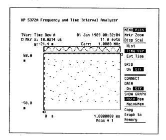
Figure 8. The first view of the measured jitter is obtained after selecting Graphic Results and picking Time Variation as the type of analysis. A calibrated display of jitter amplitude versus time, with several menus further enhances analysis.
