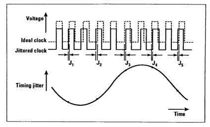
Figure A. Jitter is the deviation of the clock edges from their ideal positions in time.
