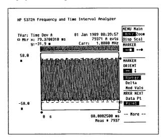
Figure 16. Choosing the maximum number of samples is not always a good default choice to make. Here are 8000 samples of jitter versus time. It is hard to identify patterns and takes longer.
