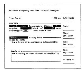
Figure 4. With the Function field highlighted, you can cycle through many choices by pressing the -- More-- key. Here, Time Deviation is selected.
