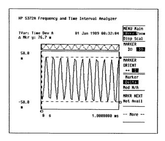
Figure 12. The peak-peak value of jitter is measured when the Delta between cursors is selected. Note the result in the upper left corner of the display.
