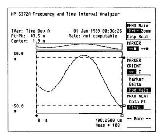
Figure 14. If you sample too fast, you will not get results that you recognize. Here you see about one cycle of jitter. Ten times faster sampling would have shown you only a small segment of the jitter.
