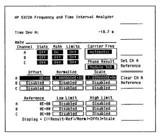
Figure 7. Several Math functions are available to be selected on the screen presented after pressing the Math hardkey. Here Automatic calculation of the clock's frequency is selected, and the results are scaled to Unit Intervals by multiplying the measured time by the clock frequency.
