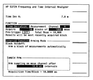
Figure 18. For statistical analysis such as a histogram, select some large number of measurements. Here 10 blocks of 1000 or 10,000 measurements are selected.
