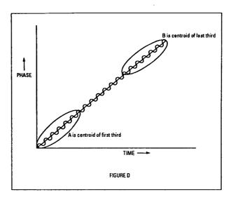
Figure D. The bi-centroid algorithm is a precise and efficient algorithm for deriving the underlying clock frequency of a modulated signal. The mean of the first and last third of the data points is calculated. The straight line joining the two means is the estimated clock frequency.
