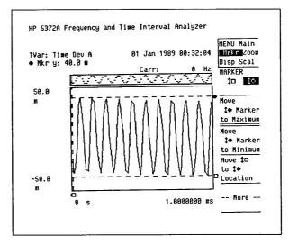
Figure 11. The next step is to move the  $\[ \] \bullet$  marker to the maximum of the waveform.
