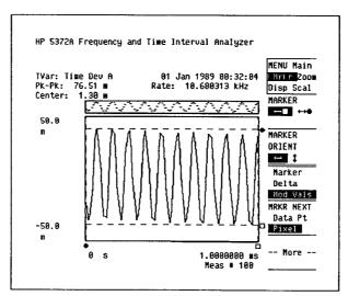
Figure 13. The HP 5372A automatically calculates modulation values if the signal is strongly periodic. Move the → cursors to either side of the waveform section of interest and both peakpeak jitter and jitter rate (frequency) are displayed at the top of the screen.
