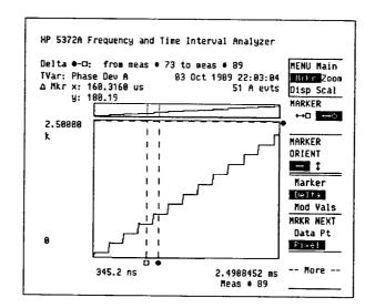
Figure 4b. Cumulative phase deviation of a BPSK signal.
