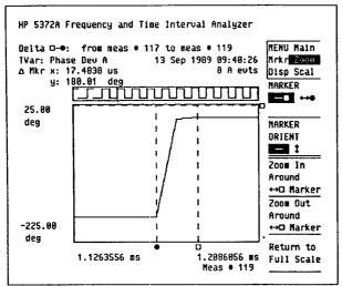
Figure 2. An individual phase change of 180.01 degrees on the HP 5372A.
