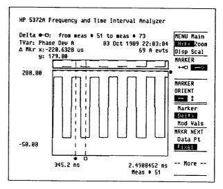
Figure 4a. Modulo 360 phase deviation of a BPSK signal.
