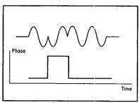
Figure 1. Time domain view of a BPSK signal and corresponding phase vs. time plot.
