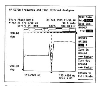
Figure 5. Example display of "wrap-around" effect with modulo 360.
