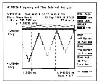
Figure 26. Phase deviation versus time in cumulative format.
