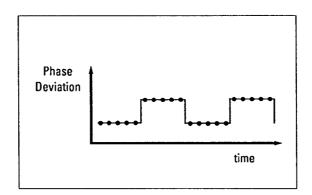
Figure C. Phase deviation plot shows phase modulation.
