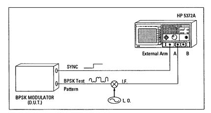
Figure 6. Typical equipment setup to measure a downconverted BPSK signal.
