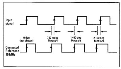
Figure 3. Simplified view of the phase deviation measurement.
