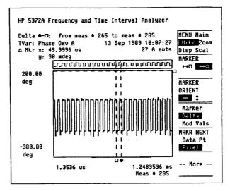
Figure 18. Dolta  $\bullet$  -  $\square$  marker indicates phase modulation interval of 49.9996  $\mu$ s.
