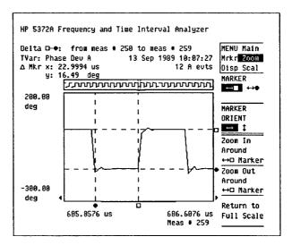
Figure 22. Digital zero phase duration is less than the desired 25  $\mu$ s.
