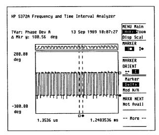
Figure 19. Delta I marker indicates overall phase change size of 180.56 degrees.
