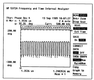
Figure 16. Phase deviation versus time with CONNECT DATA On selected.
