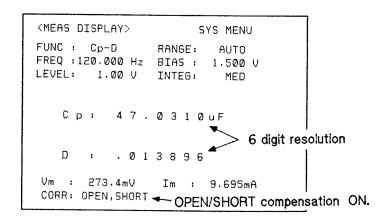
Figure 1. Highly Accurate 6 Digit
