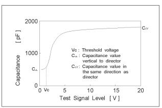
Figure 2. Voltage-capacitance Characteristics Measurement Results
