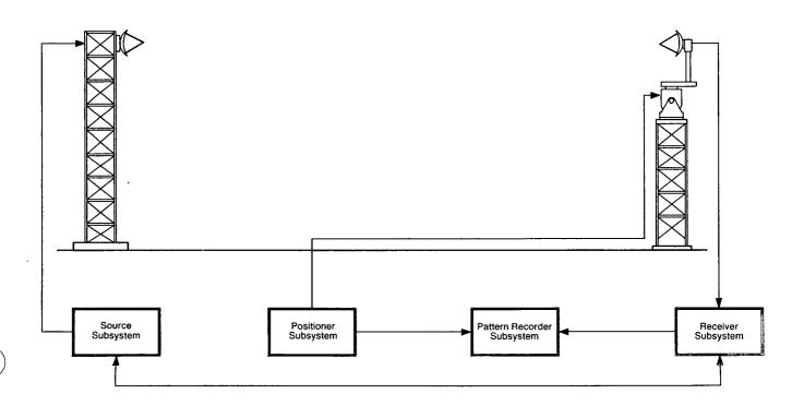
Figure 1. Typical Antenna Test System Block Diagram
