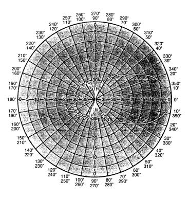
Figure 7. E-plane 40 dB Polar Plot of a Conical Broadband Horn at 8.5 GHz
