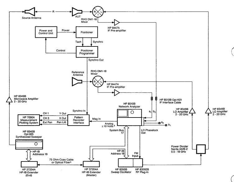
Figure 5. Detailed Hookup Diagram of External Phase-lock Configuration
