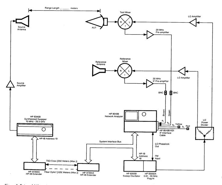
Figure 3. External Mixer Antenna Test System
