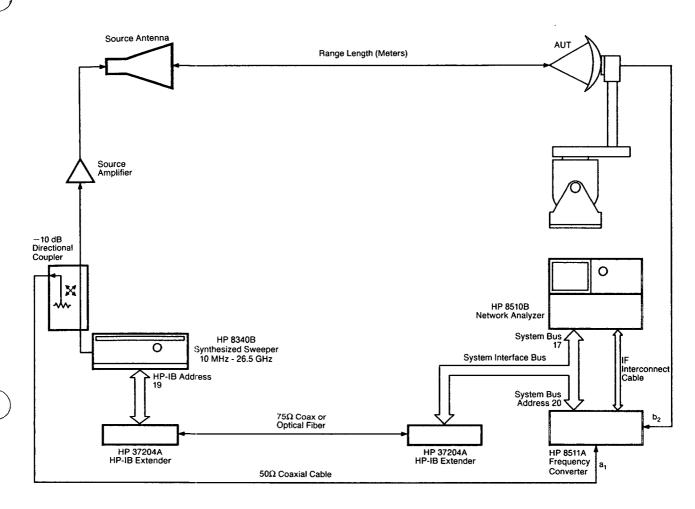
Figure 2. Antenna Test System Using an HP 8511A Frequency Converter
