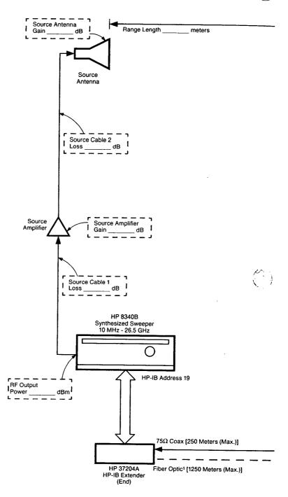
Figure A-2. Power Budget Worksheet for External Mixer Configuration
