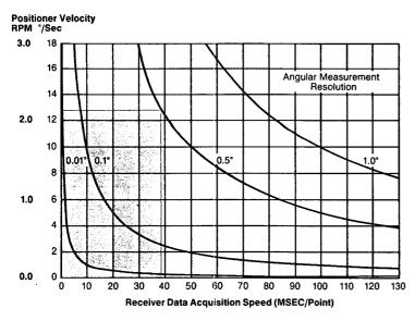
Figure 4. Positioner Velocity -vs- Acquisition Rate and Angular Resolution
