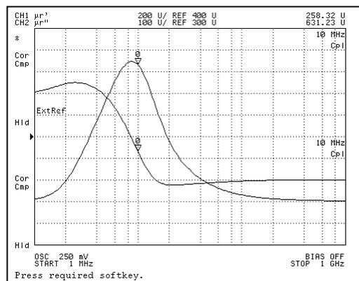
Fig.33 Frequency Response of MnZn Ferrite Core
