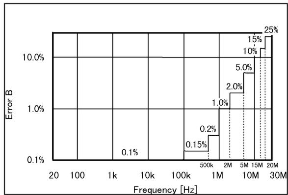
**Fig.42 Relative Measurement Accuracy**
