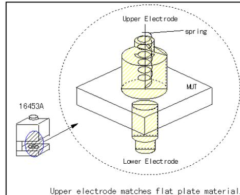
**Fig.18 Structure of 16453A**
