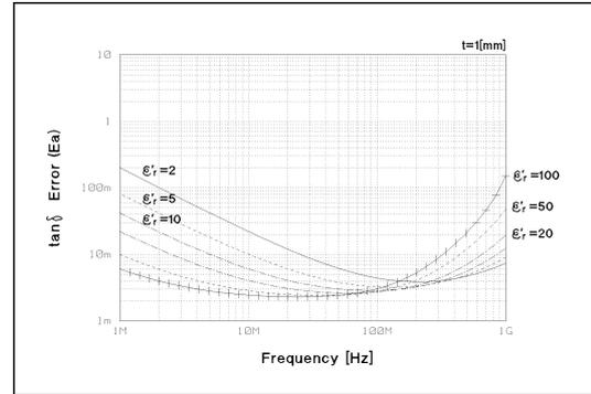
**Fig.20 Loss Tangent Measurement Accuracy (Supplemental Data)**
