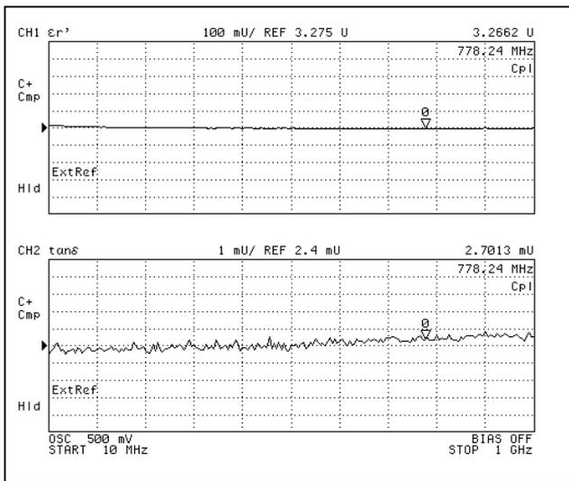
**Fig.24 Frequency Response of BT Resin**
