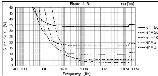
**Fig.12 Permittivity Measurement Accuracy**
