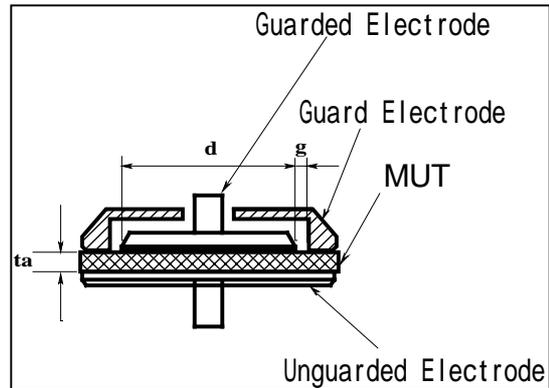
**Fig.4 Contacting Electrode Method**
