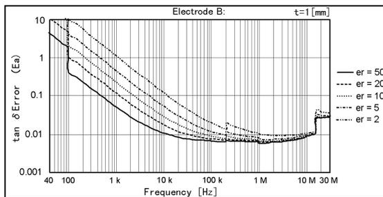
**Fig.13 Loss Tangent Measurement Accuracy**
