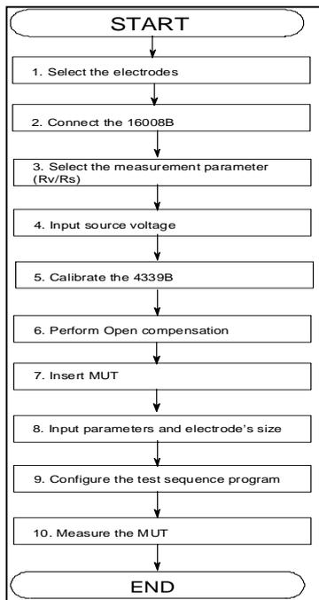
**Fig.39 Measurement Procedure Flowchart for the 4339B and the 16008B**
