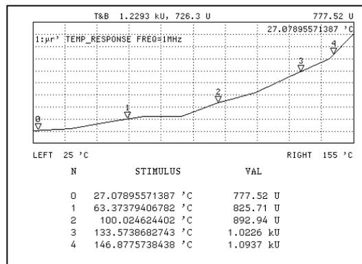
Fig.34 Temperature Response of MnZn Ferrite Core
