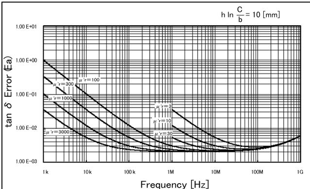
**Fig.31 Loss Tangent Measurement Accuracy (Supplemental Data)**
