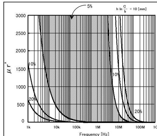
Fig.30 Permeability Measurement Accuracy (Supplemental Data)
