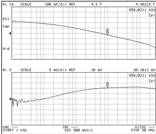
**Fig.15 Frequency Response of Printed Circuit Board**
