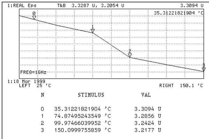
**Fig.25 Temperature Response of BT Resin**
