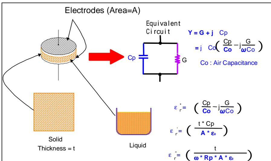
Fig.2 Parallel Plate Method
