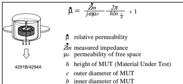
Fig.29 Structure of 16454A and Measurement Concept
