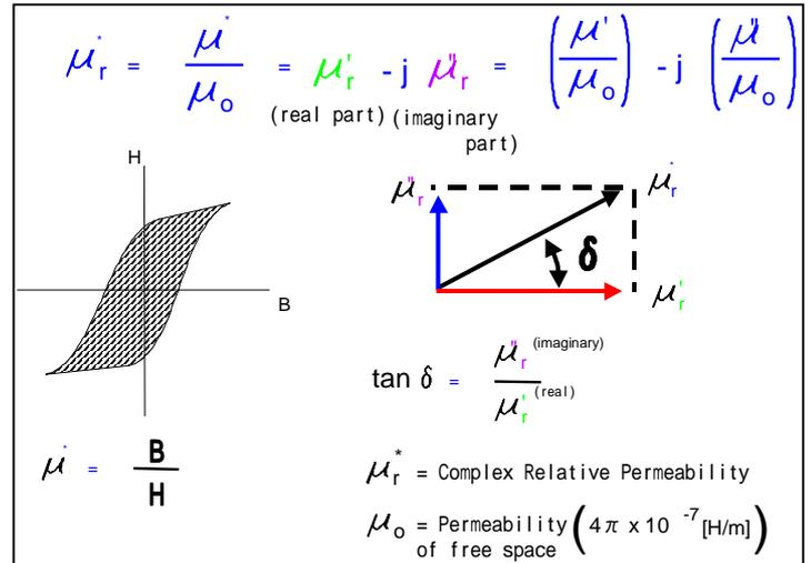
**Fig.26 Definition of Complex Permeability ( $\mu^*$ )**
