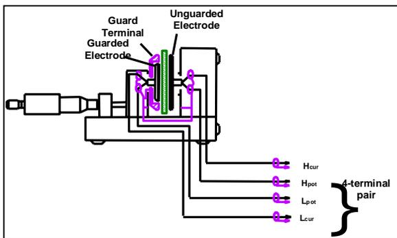
**Fig.11 Structure of 16451B**
