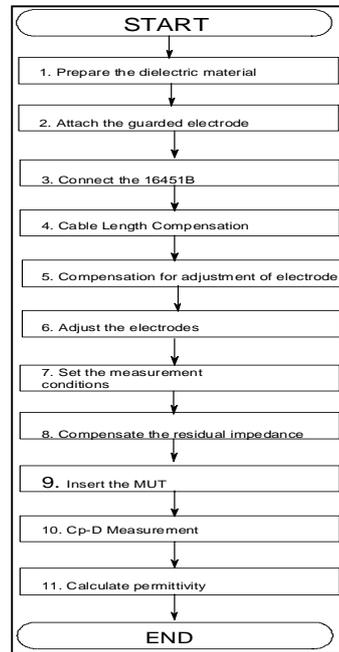
**Fig.14 Measurement Procedure Flowchart for the 16451B**
