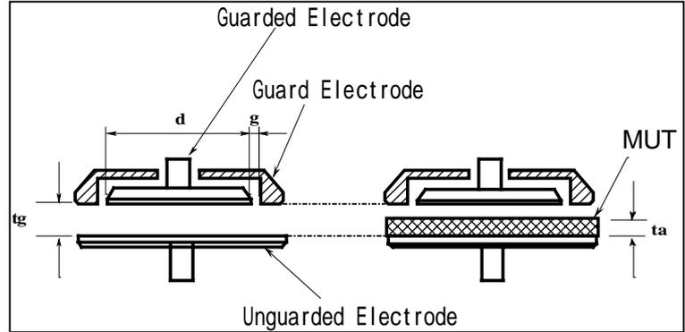
**Fig.6 Non-Contacting Electrode Method**
