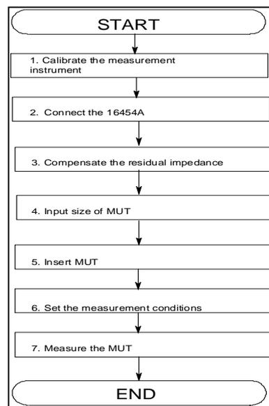
**Fig.32 Measurement Procedure Flowchart for the 16454A**
