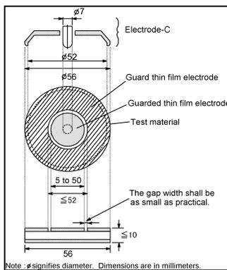
**Fig.9 Electrode C Dimensions**
