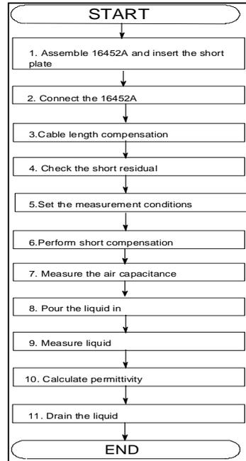
**Fig.43 Measurement Procedure Flowchart for the 16452A**
