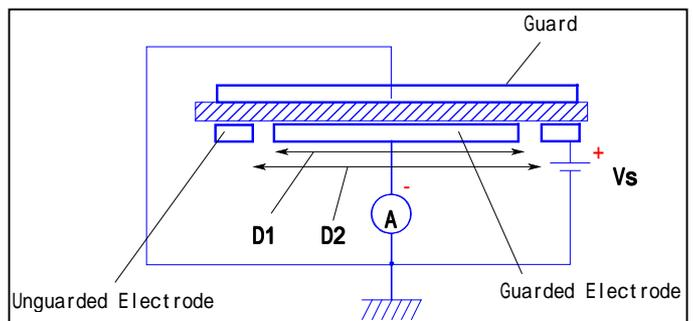
Fig.37 Surface Resistivity
