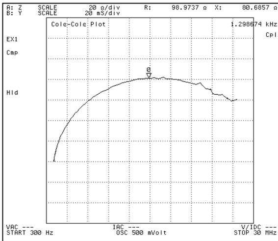
**Fig.16 Cole-Cole Plot of a Ceramic Material**
