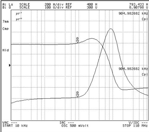
**Fig.35 Frequency Response of MnZn Ferrite Core**
