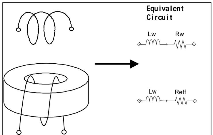
**Fig.27 Method of Measuring Effective Permeability**
