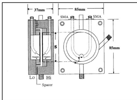
**Fig.41 Structure of 16452A**
