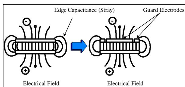
**Fig.3 Effect of Guard Electrode**
