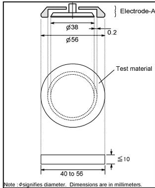
**Fig. 7 Electrode A Dimensions**
