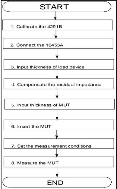
**Fig.21 Measurement Procedure Flowchart for the 16453A**
