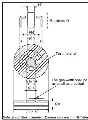
**Fig.10 Electrode D Dimensions**
