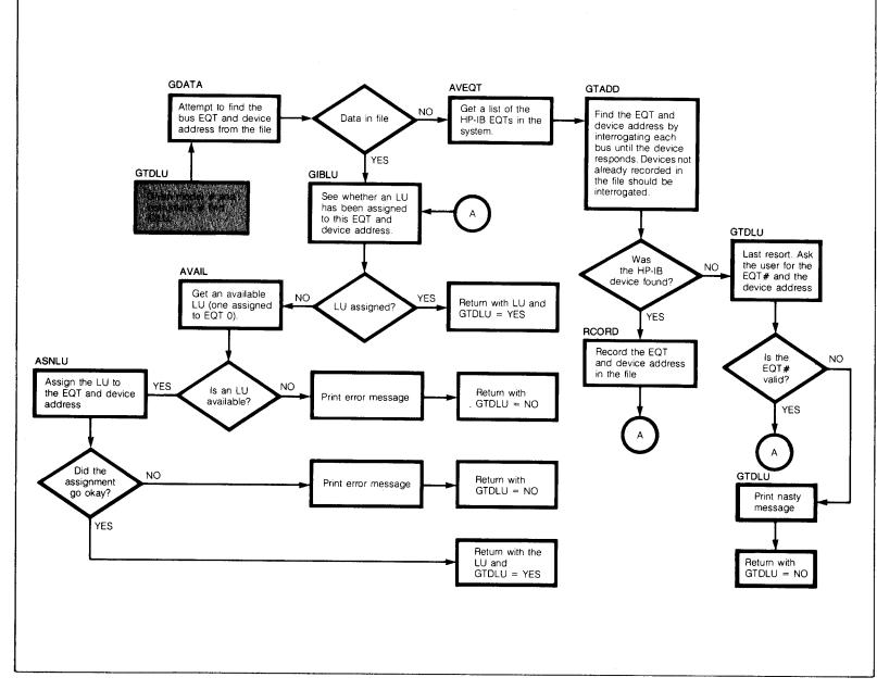
Figure 6-5. Flowchart Showing the Steps Required for HP-IB LU Determination Using GTDLU
