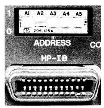
Figure 1-4. A Typical Set of Address Switches
