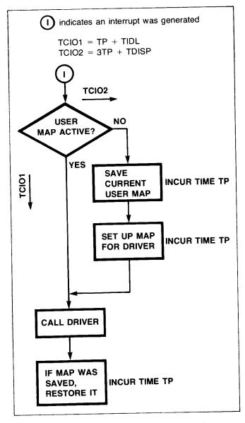
Figure 4-5. Flowchart of Map Switching Time
