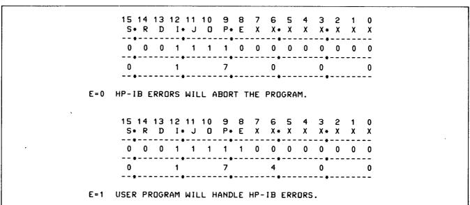
Figure 15-2. Example Device Configuration Words
