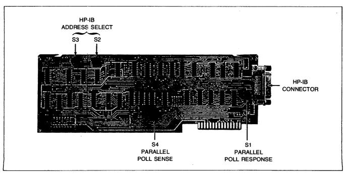
Figure 15-1. Layout of the A2A9 Printed Circuit Board
