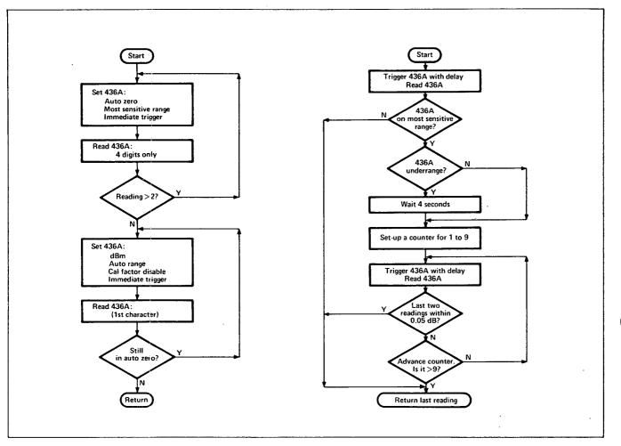
Figure 16-5. Flowchart for 436A Device Subroutines
