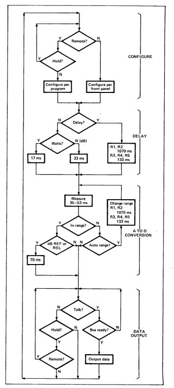
Figure 16-7. Flowchart for 436A Internal Timing
