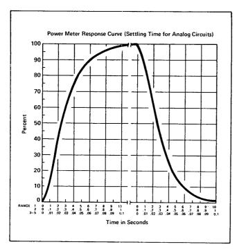
Figure 16-8. Settling Time for Power Meter Ranges
