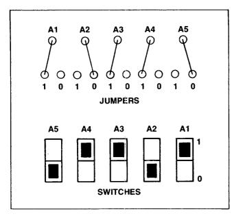
Figure 16-2. HP-IB Switch or Jumper Positions
