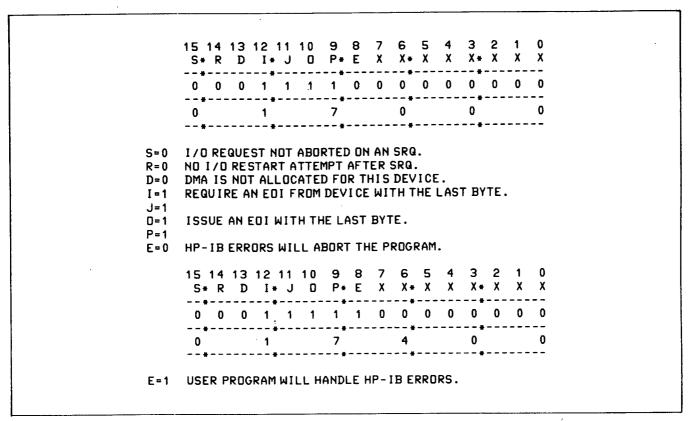
Figure 17-3. Example Device Configuration Words
