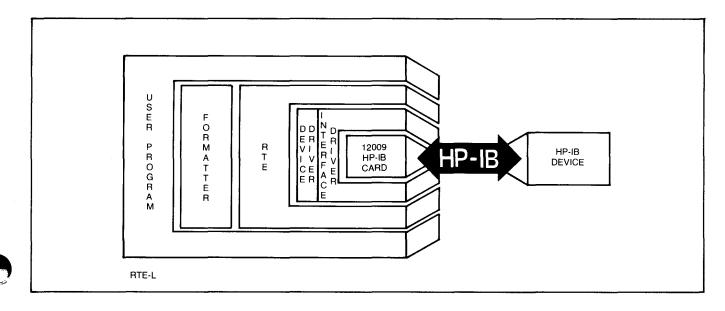
Figure 1-4. Software/Hardware Interface
