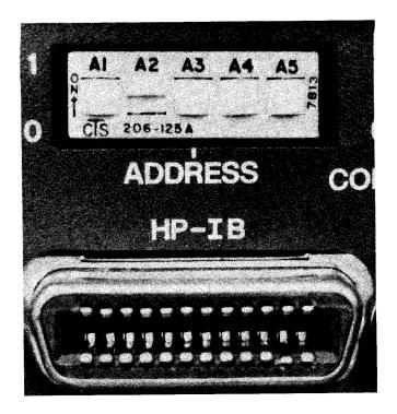
Figure 1-2. A Typical Set of Address Switches
