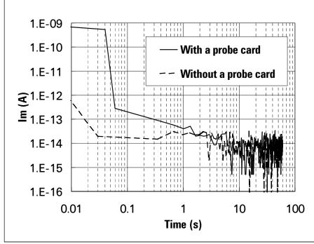
Figure 9. 4073A settling characteristics (when 100 V is applied)
