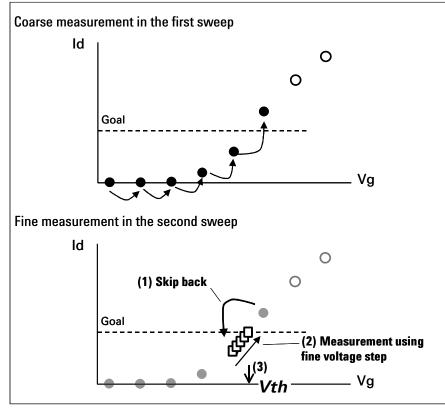
Figure 7. Vth measurement using intelligent search
