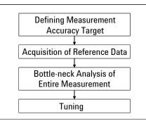
Figure 4. Flow of throughput tuning
