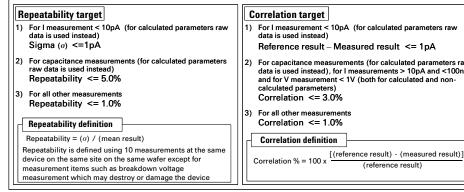
Figure 5. Example definition of measurement accuracy target
