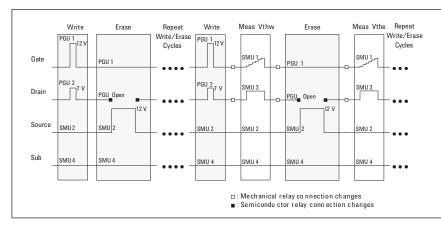
Figure 6. NOR Type Flash Memory Write/Erase Cycles Test Timing Chart
