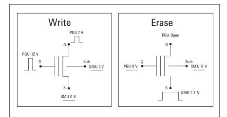
Figure 2. Typical Write and Erase Pulses for NOR Type Flash Memory Cell
