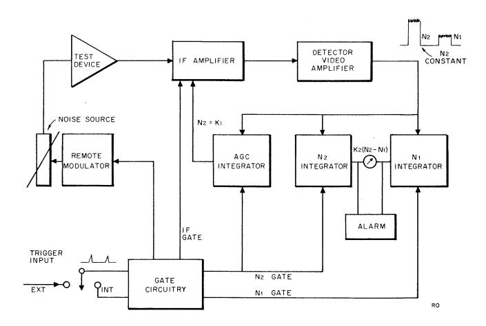
Figure 4. @ 344A Noise Figure Meter Block Diagram
