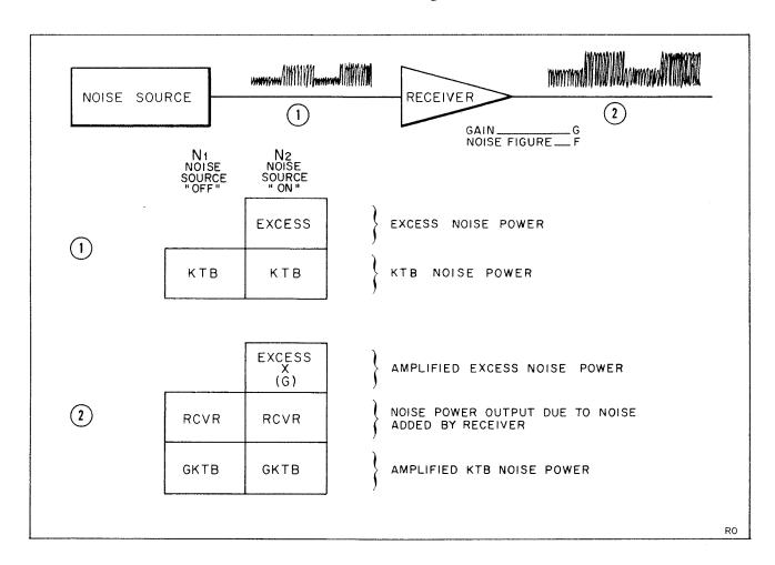
Figure 1. Automatic Noise Figure Measurement of Microwave Device (Composition of Noise Power)
