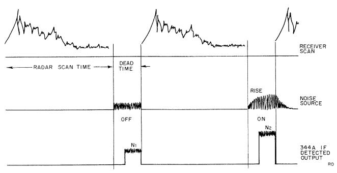
Figure 3. Timing Relations for the System shown in Figure 2
