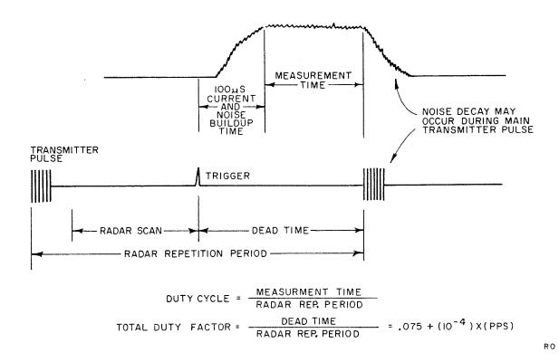
Figure 5. 344A Measurement Duty Cycle Requirements
