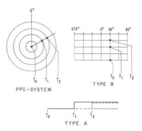
Figure 7. Radar System Calibration
