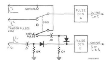
Figure 10. Triple Pulse Generator
