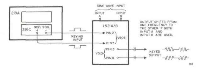
Figure 9. Using the 218A/219C with the 152A/B Oscilloscope Plug-In to Provide Pulse Bursts or Frequency Shift Keying
