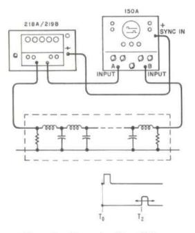
Figure 5. Measuring Time Delays
