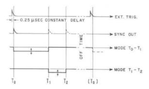
Figure 3. Time Plan, 219C Plug-In Unit
