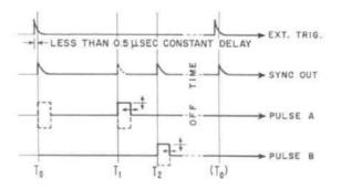
Figure 2. Time Plan, 219B Plug-In Unit
