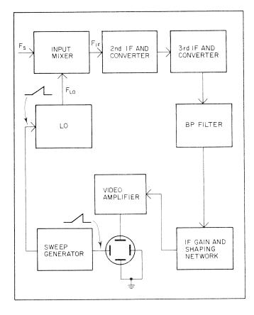
Figure 13. Functional Block Diagram
