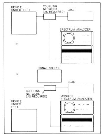
Figure 7. Conducted EMI Tests
