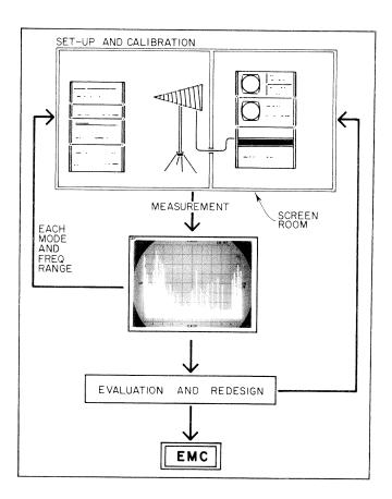
Figure 3. EMI Measurement Flow Chart
