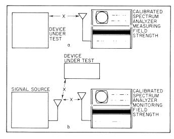
Figure 4. Radiated EMI Tests
