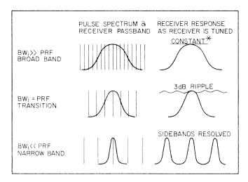
Figure 11. Receiver Response to a Pulse
