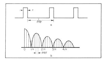
Figure 10. Pulse Spectrum
