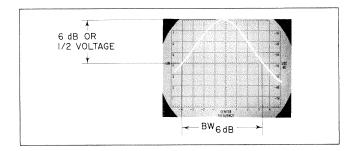
Figure 15. Measurement of 6-dB Bandwidth
