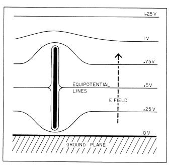
Figure 6. Derivation of Antenna Factor for 1 Meter Rod
