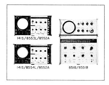
Figure 12. HP Spectrum Analyzers
