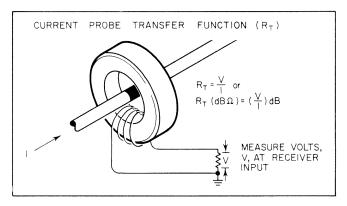
Figure 8. Current Probe Transfer Function
