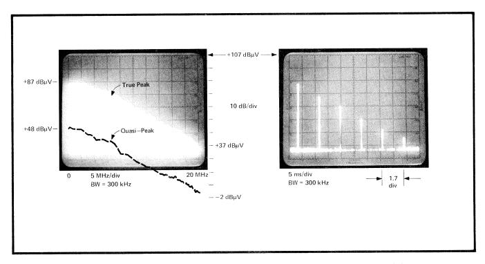
**FIGURE 1.** (a) This is the true peak of conducted EMI from an SCR light dimmer, and the quasi-peak level found from the graph. (b) The PRF is determined by video triggering and using the calibrated scan time to determine the time between pulses.
