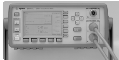
Figure 6. E4417A power meter configured to show a trace display (upper window) and a dual numeric display (lower window).
