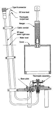
Figure 2. Schematic cross-section of the NIST coaxial microcalorimeter at Boulder, Colorado, U.S.A.
