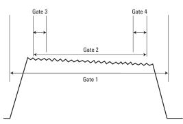
Figure 12. On this GSM pulse, powerful data configuration routines during four gate times, provide the feeds for the display.
