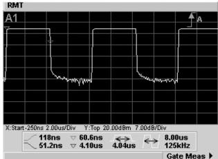
Figure 8. Large color display with automatic power and time measurements
