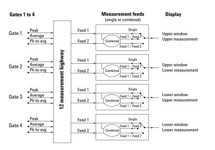
Figure 15. User-configured data manipulations are one big feature of the EPM-P series power meters.
