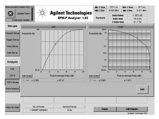
Figure 14. The Y-axis shows the percent time the signal power is at or above the power specified by the X-axis.
