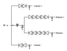
Figure 5. Simplified block diagram of the twopath-diode-stack topology.
