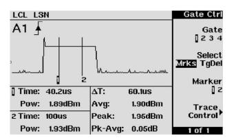
Figure 13. This graphical display permits marker-selected power measurements, plus computations between the marker-identified data.
