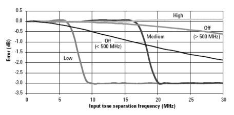
Figure 7. N192XA Error in peak-to-average measurements for a two-tone input (High, Medium and Low or Off video bandwidth)
