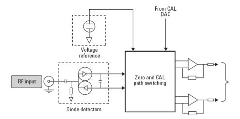
Figure 6. Internal zero and cal block diagram
