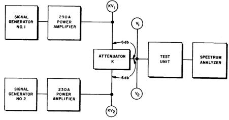
Figure 6. Connections for Checking Small Amounts of Intermodulation
