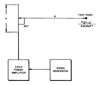
Figure 13. Using Radiated Signals
