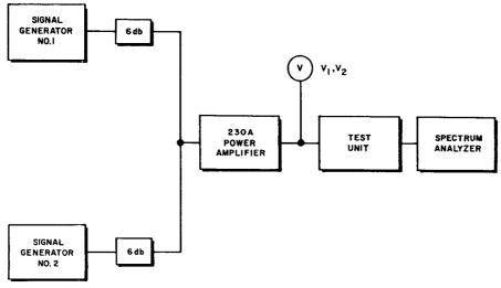
Figure 4. Connections for Checking More than 2% Intermodulation
