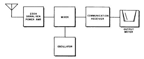
Figure 16. Setup for Leakage Testing
