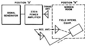
Figure 11. Setup for Screen Room Testing
