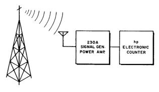
Figure 15. Setup for Remote Frequency Monitoring
