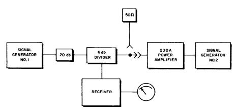
Figure 2. Connections for Desensitization Test
