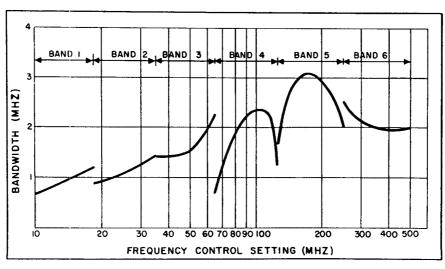
Figure 12. Typical Bandwidth vs. Frequency Curves for the 230A
