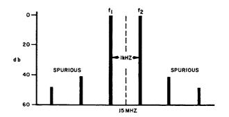
Figure 3. Spectrum for Analyzing Amount of Intermodulation
