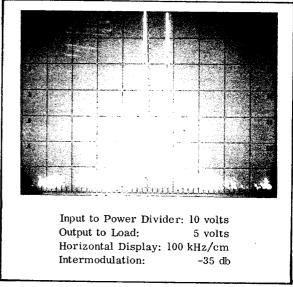
Figure 7. Spectrum Displays, Intermodulation
