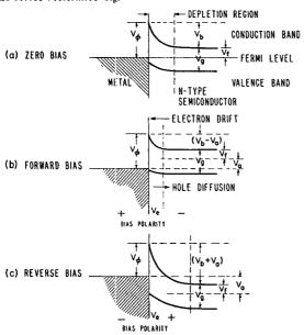
Figure 3. Energy Level Diagram for Hot Carrier Diode  $V_{\phi} =$  Barrier Potential. A constant depending on the metal  $V_{b} =$  Built-in Potential  $= V_{\phi} - V_{f}$   $kT = N_{c} \qquad N_{c} = \text{Effective Density of states in}$
