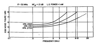
Figure 17. Typical Noise Figure vs. Frequency  $P_{LO} \equiv 1 \text{ mW}$ .  $f_{IF} \equiv 30 \text{ MHz}$ .  $NF_{IF} \equiv 1.5 \text{ dB}$
