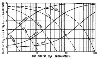
Figure 14. Optimum Bias for Specified Frequency (f) and Amplifier Noise Resistance (R<sub>A</sub>)
