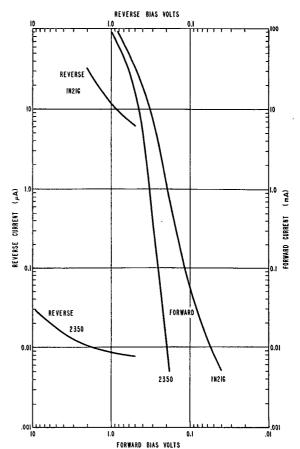
Figure 9. Forward VI Characteristics
