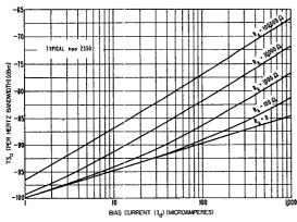
Figure 12. Variation of TS<sub>o</sub> with Bias Current Typical HPA 2350
