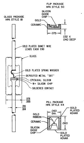
Figure 5. Cross-Sections of Hot Carrier Diodes
