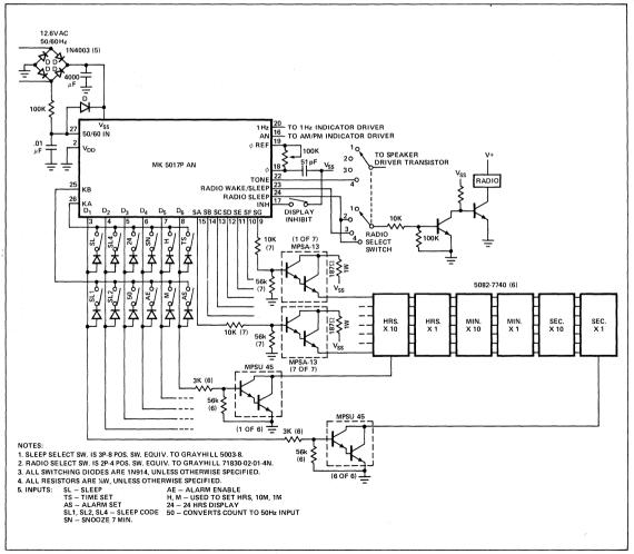
Figure 7. Six Digit Clock Radio.
