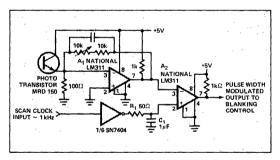
Figure 11. Wide Dynamic Range Intensity Control Circuit.
