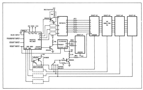
Figure 8. Four and One-half Digit Strobed Counter
