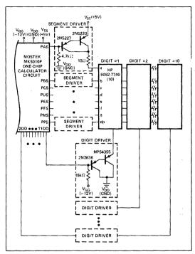
Figure 5. Typical Single Chip Calculator Circuit.
