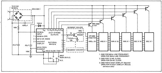
Figure 6. Strobed Drive for a Six Digit Clock.
