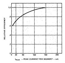
Figure 2a. Relative Efficiency (Luminous Intensity per Unit Current) versus Peak Current per Segment.
