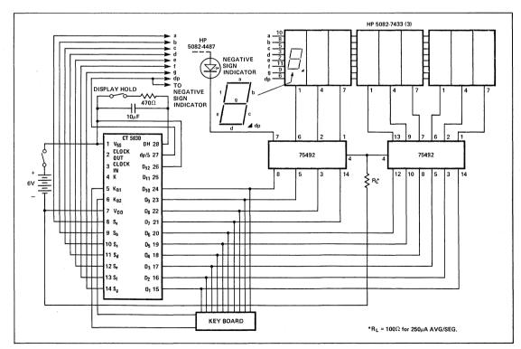
Figure 5. Four Function Calculator.
