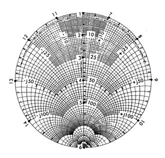
Fig. 4 — Points on the r plane (r defined by Equation 3) identified for location on the s plane for the series and shunt mapping. Note the circles which go through 1-6, 2-6, 3-6, 4-6 and 5-6 are constant r circles, while those through 7-6, 8-6, 9-6 and 10-6 are constant inductive reactance circles and the corresponding circles through 11-6, 12-6, 13-6 and 14-6 are capacitive reactance circles.
