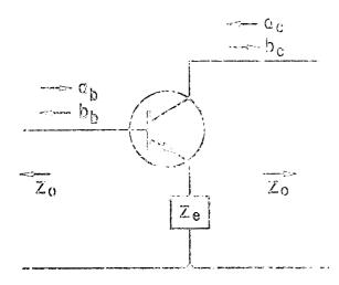
Fig. 2 — Incident and reflected waves for a transistor in common emitter configuration with an arbitrary impedance Z<sub>e</sub> in the emitter lead.
