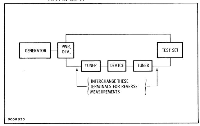
Figure 4. Setup for Measuring MSG, GMAX, K, U
