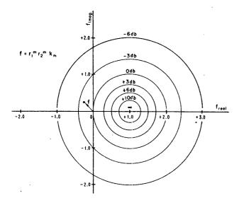
Fig. 8 - Constant gain circles giving contribution total transducer panel gain due to interaction term  $G_{12m}$  as a function of the generator r<sub>1</sub>m, the load r2m and the device k<sub>m</sub>.
