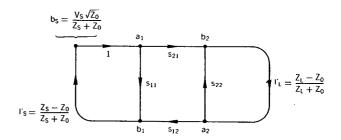
Fig. 3. Flow graph of network of Fig. 2.
