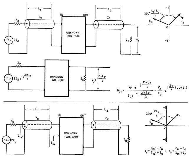
S parameters can be measured remotely. Top test setup is for measuring  $s_{21}$ ; bottom, for  $s_{11}$ . Measured vector  $V_2/E_0$  is the voltage transducer gain of the two-port and cables  $L_1$  and  $L_2$ . The measured vector  $r_1$  is the reflection coefficient of the two-port plus input cable  $L_1 + L_2$ . Appropriate vectors for  $r_1$  and s parameters are plotted.
