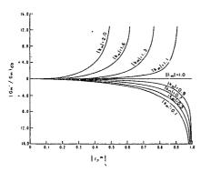
Fig. 6(a) — Set of curves giving the radii of constant power gain circles as a function of the load  $|\mathbf{r}_2^{\mathbf{m}}|$  with  $|\mathbf{k}_{\mathbf{m}}|$  as a parameter. This set of curves provides circles of positive power gain for K > 1.
