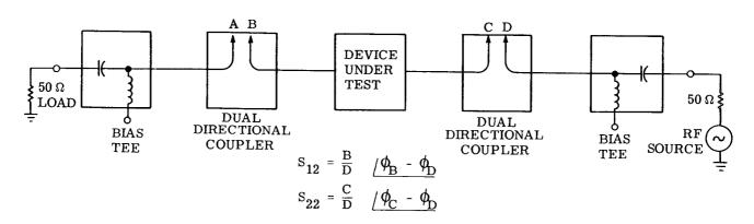
These circuits can be constructed from individual components or supplied in a single box. When the circuit is contained in a single box, the tedious job of connecting coax circuitry disappears, and s-parameter measurements can be made by pushing a button. This is the case with the HP 8745A S Parameter Test Set.
