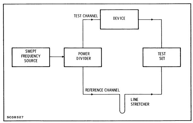
Figure 2. Setup for Measuring  $\mathbf{S}_{12}$  and  $\mathbf{S}_{21}$
