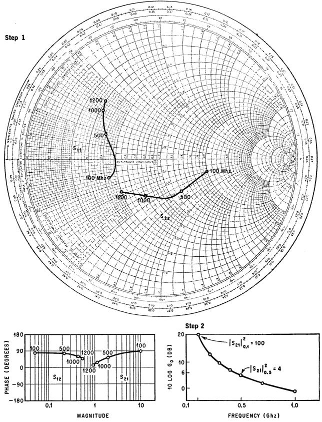
From the measured data transducer power gain is plotted as decibels versus frequency. From the plot an amplifier of constant gain is designed. Smith chart is used to plot the scattering parameters.
