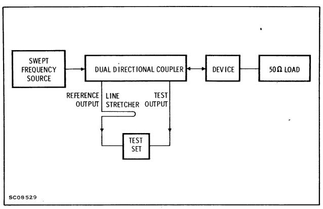
Figure 3. Setup for Measuring  $\mathbf{S}_{11}$  and  $\mathbf{S}_{22}$
