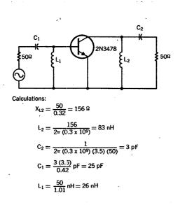
Fig. 7. 300-MHz amplifier with matching networks for maximum power gain.
