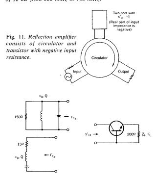
Fig. 12. Transistor oscillator is designed by choosing tank circuit such that  $\Gamma_T s'_{11} = 1$ .
