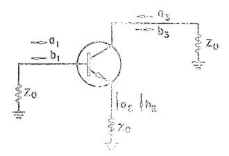
Fig. 1 — Incident and reflected waves (a, b respectively) for a transistor imbedded in a structure where all three leads are terminated by the characteristic impedance  $\mathbf{Z}_0$  of a transmission line.
