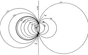
Fig. 10 - Constant gain circles (g<sub>o</sub>) for a set of s parameters which satisfy case C of Fig. 9. Gain g<sub>2</sub> is given as a numerical ratio, not ₫B. Circles are plotted on the r<sub>2</sub> plane. s<sub>11</sub> ==  $0.707 / 0^{\circ}; s_{22} = 0.707 / 0^{\circ}; s_{12}$  $s_{21} = \overline{0.2} / 0^{\circ}$ .
