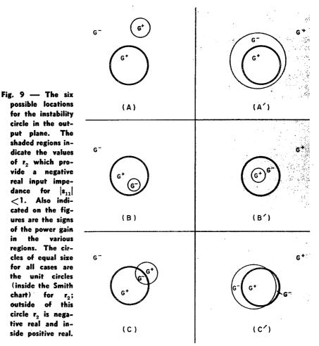
9(A) Input unconditionally stable; simultaneous matched load positive real.  $|r_2^m| < 1;$ k > 1;  $D_2$  positive;  $k_m < 1$ .
