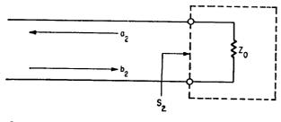
By setting  $a_2$  equal to zero the  $s_{11}$  parameter can be found. The  $Z_0$  resistor is thought of as a one-port network. The condition  $a_2=0$  implies that the reference impedance  $R_{02}$  is set equal to the load impedance  $Z_0$ . By connecting a voltage source,  $2 E_{01}$ , with the source impedance,  $Z_0$ , parameter  $s_{21}$  can be found using equation 5
