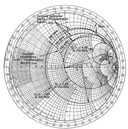
Fig. 8. Smith Chart for broadband amplifier design example.
