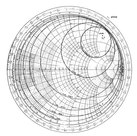
Fig. 4 — Contours of constant gain  $G_1$  and constant  $|\mathbf{s}_{11}|$  indicating gain and match obtained for various generators  $r_1$ .  $|s_{11}|$  was taken as 0.867 at  $-45^{\circ}$ .
