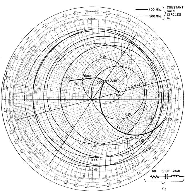
Load impedance is found by inspecting the output plane for loci that give proper gain.
