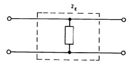
8. Add emitter feedback to device with shunt feedback,  $Z_{T2} = Z_{R} + Z_{T1}$ .
