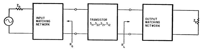
To design an amplifier stage, source and load impedances are found to give the gain desired. Then impedances are synthesized, usually as matching networks between a fixed impedance source or the load and the device. When using s parameters to design a transistor amplifier, it is advantageous to distinguish between a simplified or unilateral design for times when s<sub>12</sub> can be neglected and when it must be used.
