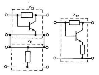
9. Convert Z matrix of device with feedbacks to X matrix,  $Z_{T2} \rightarrow X_{T1}$ .
