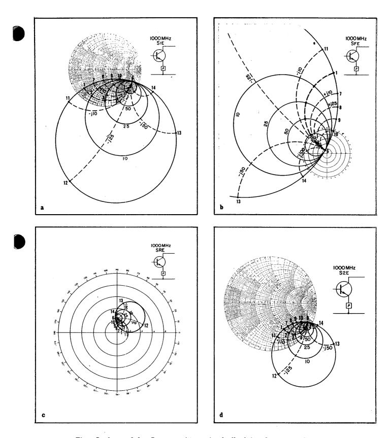
Figs. 5a, b, c and d — Common emitter series feedback impedance mapped onto the s-parameter planes at 1 GHz. The shaded regions correspond to inductive impedance while the colored areas are capacitive.
