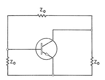
Fig. 3 — A three-terminal device imbedded in a network which can be used to readily evaluate the effects of shunt feedback.
