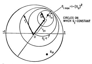
A graphical plot helps in design of an amplifier stage. Here the measured parameters  $s_n$  and  $s_n^*$  are plotted on a Smith chart. The upper point is  $s_n^*$ .
