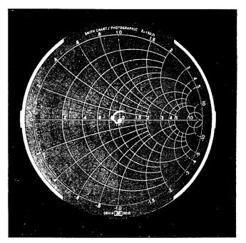
venience of polar display and swept measurement, you can get by with just the Vector Voltmeter (HP 8405, \$2750), top of the shelf to the left. It will work up to 1 GHz. A photo of a Smith chart overlay (white grid) of  $S_{22}$  over a 100 to 400 MHz range obtained by the author, Les Besser, is shown on the right.
