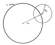
Fig. 3 — Circle defined by  $\mathbf{r}_{s2}$  and  $\rho_{s2}$  divides  $\mathbf{r}_{2}$  plane into a stable and potentially unstable region of operation. If  $|\mathbf{s}_{11}| < 1$ , the inside of the circle indicates those loads which provide negative real input impedance  $(|\mathbf{s}_{11}'| > 1)$ . The heavier weight circle defines the unit circle on the Smith Chart.
