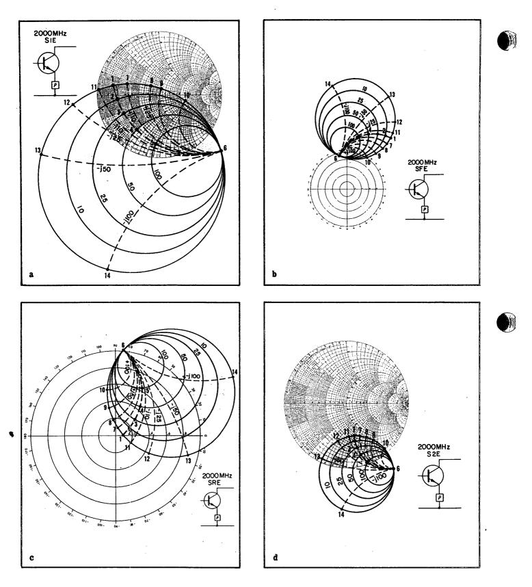
Figs. 6a, b, c and d — Common emitter series feedback impedance mapped onto the s-parameter planes at 2 GHz. The shaded regions correspond to inductive impedances while the colored areas are capacitive.
