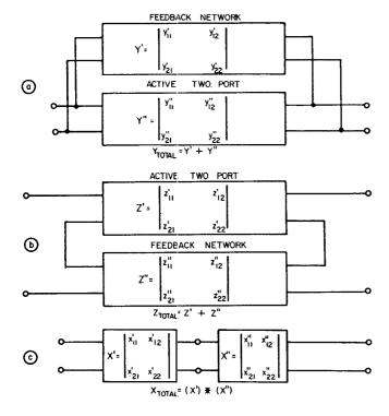
1. Feedback is added and two-port networks are cascaded by means of admittance (a), impedance (b) and modified transmission (c) parameters. See text for the derivation of the X-parameter matrix.
